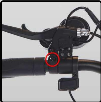
Check whether the brake lever screws are tightened.
