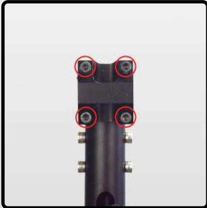
① Loosen the screws on the handle mount with a 4mm hex wrench, which is included in the basic tool kit.
