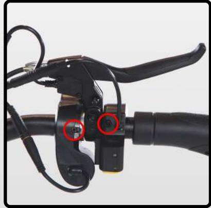
Make sure the voltage lock and light button screws are tightened.
