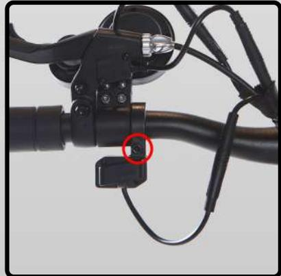
Check whether the SINGLE/DUAL button screws are tightened.
